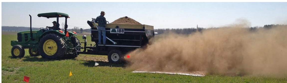
Figure 1. Spreader calibration for a poultry litter field application.
